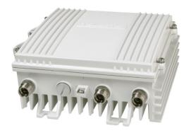
The AC3210 is a dual active output amplifier with 48 dB maximum gain. The amplifier stages are based on extreme high performance GaN solution that makes the usable gain range especially wide and allows high output level. Integrated interstage gain and slope controls optimise the flatness performance.
