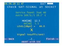
One of the wizards: simple and guided check of the signal quality at the antenna socket.
